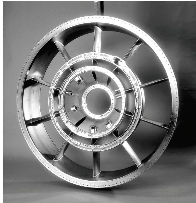
Figure 8. One piece titanium Ti-6-4 investment casting after HIP-ing, \alpha -case removal by chemical milling and machining to final dimensions. BR 715 front fram.
