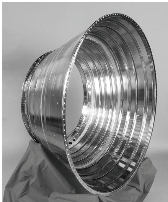
Figure 15. A low pressure turbine casing for the LM 6000 engine made by joining two ring rolled parts with a circumferential EB-weld at the center discerned by the etched grayish appearance. The front small diameter part is made of alloy 718 while the aft part is made of the higher temperature capacity Waspaloy alloy.
