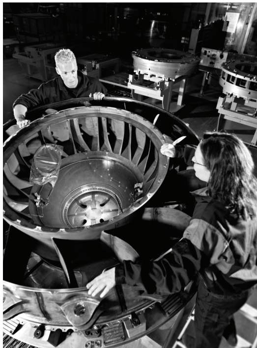
Figure 14. Alloy 718 structural parts which combines wrought and cast material. The upper part is a compressor rear frame for the GE CF6 engine while the lower is a turbine rear frame for the new GENx engine.
